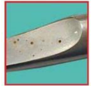
Chloride-induced pitting on instrument.
